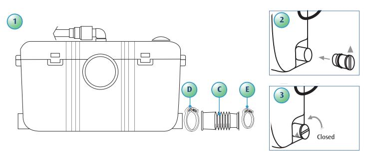
To connect to the side entries of the case, use the rubber connector (C). Secure with plastic clips (D) and (E). Plug the unused inlet with blanking plug (F) after greasing the joint.
