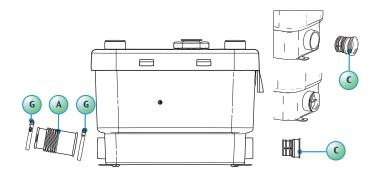
Use the rubber connector (A) for connection of pipes to the side inlets.
