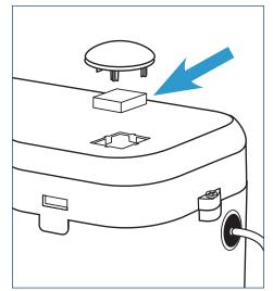
Sanibest is fitted with an active carbon filter, and requires no external venting.
