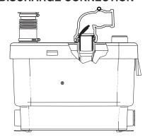
Note: The discharge pipework should be 32mm copper or rigid solvent weld plastic.
