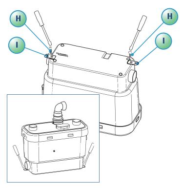
The unit should be accessible for possible maintenance. It is supplied with floor fixing lugs to prevent it from moving during
