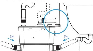
For possible service requirements, provide a drain off at the low point of the installation.
