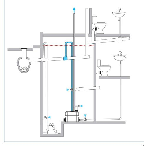
50mm discharge outlet. The Sanicubic will not be able to operate at all if this vent connection is not opened up!
