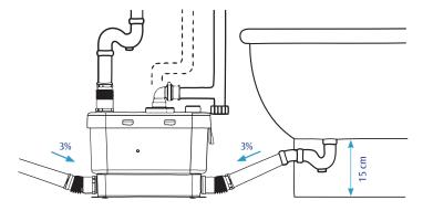
To connect a shower/bath, ensure that the trap exit is 15cm above floor level. Although not obligatory, a lid connection may be used to run an external air vent.
