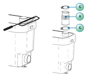
To connect to a lid inlet, cut off the sealed cap with a hacksaw and connect using the rubber connector (A) provided. Tighter with the metal hose clips (G).
