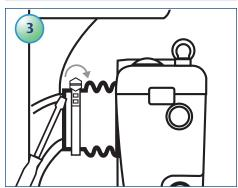
Pull flexible sleeve over the pan spigot (fig 1) Position the jubilee clip over the edge of the flexible sleeve (fig 2), and tighten with a screwdriver (fig 3).
