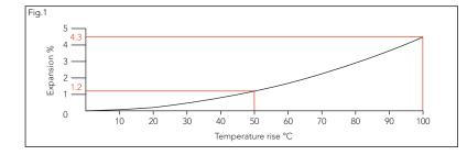
With unvented systems there are no cistern tanks or open outlets to accommodate expansion. All systems above 15 litre, and some systems of 15 litre or less, employ an expansion vessel or an internal air-gap to accommodate expansion.
