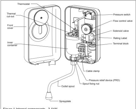
Figure 1 Internal components - 3.1kW
