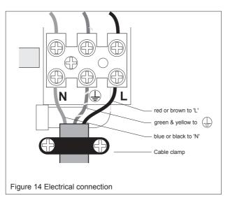
7.9 Make sure that all the terminal block screws are sufficiently tight.7.10 Refit the clamp bar.
