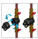
**2** Fit the flush adaptor to the port block by hand tightening the port block locking collar.
