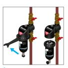
All non-magnetic contaminant is collected in the bottom of the bowl. This should be emptied and any retained contaminant should be rinsed off if necessary. Check the mesh filter in the cartridge for blockages.
