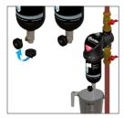
3 Using the bowl spanner provided unscrew the bowl locking collar releasing the bowl from the lid
