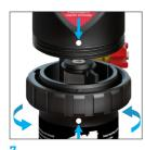
7 Check that the pre-fitted 'seal is still seated correctly. Hold the bowl to the lid ensuring the spigots on each are aligned then hand tighten the bowl locking collar.
