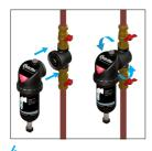
4 Ensure that the watertight seal in the filter lid opening is in place. This is supplied pre-fitted. Fit the filter body to the port block by hand tightening the port block locking collar.
