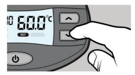
NOTE: To confirm SET temperature at any time, simply push the UP / DOWN arrow button – the display will briefly show the SET temperature before reverting back to ACTUAL temperature again.
