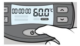
d) To set desired temperature, press the UP or DOWN arrow button and the display will show the last temperature used. To adjust, push & hold either the UP or DOWN button – the display will show the temperature changes in 0.5°C increments.
