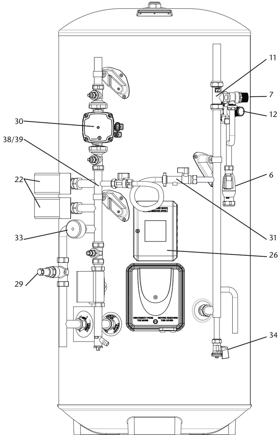
Fig 10 - Pressure Reducing valve 3.5 bar
