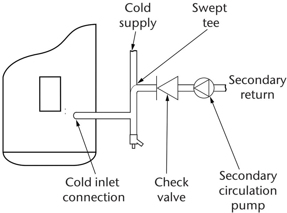
Fig 4 - Secondary circulation connection
