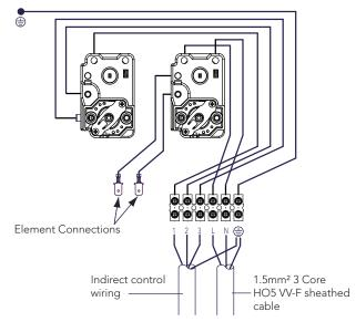
Figure 4: Indirect wiring schematic
