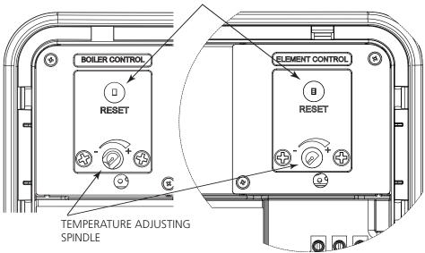
Figure 11: Thermostat adjustment
