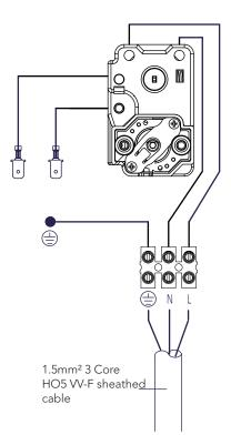
Figure 5: Direct wiring schematic
