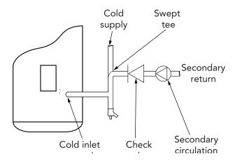
Figure 9: Secondary circulation schematic
