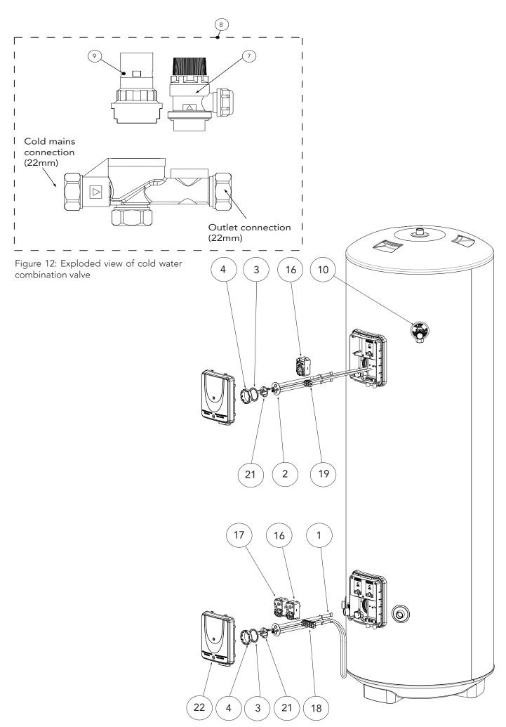
Figure 13: Cylinder exploded view
