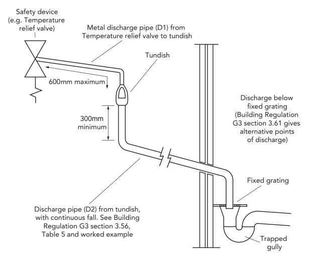
Figure 10: Typical discharge pipe arrangement (extract from Building Regulation G3 Guidance Section 3.50)
