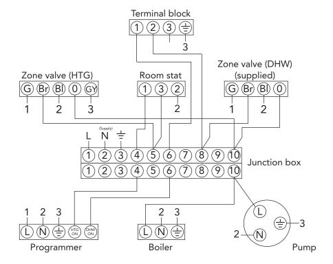
NOTES: Control terminal numbering may differ from those shown. Refer to instructions with controls selected. A double pole isolating switch must be installed in the mains supply. All earth connections must be connected back to the mains earth supply.
