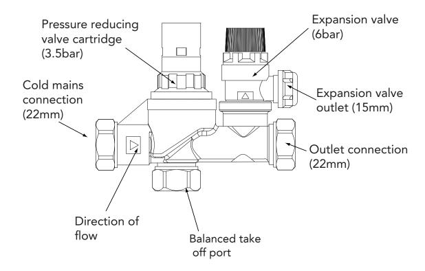
Figure 8: Combination inlet valve
