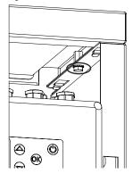
6) Slide the key holes slots in the bottom panel over the screws with star washers fitted earlier in the bottom of the side panels. Then tighten the screws complete with star washers to secure the bottom panel
