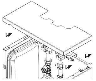
5) Fix the top panel to the right hand side panel with a M5 hex bolt and star washer using a spanner. **This is for earth continuity.**
