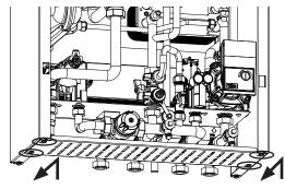
7) Fit the front panel by hooking the latches in the front panel into the holes at the front of the side panels and then pushing downwards.
