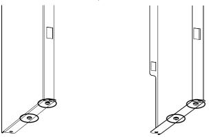
2) Fit right and left hand side panels by locating onto the hooks on the back plate and pushing downwards.
