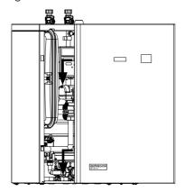
8) Fix the front panels to the lower tabs on the side panels using two M5 button head screws and star washers.
