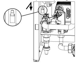
3) Fix the two side panels to the back lower tabs on the back plate using two M5 button head screws and star washers.
