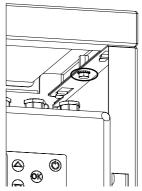
6) Slide the key holes slots in the bottom panel over the screws with star washers fitted earlier in the bottom of the side panels. Then tighten the screws complete with star washers to secure the bottom panel
