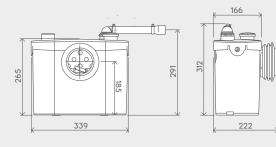
Discharge Pipework 22 / 28 / 32mm
