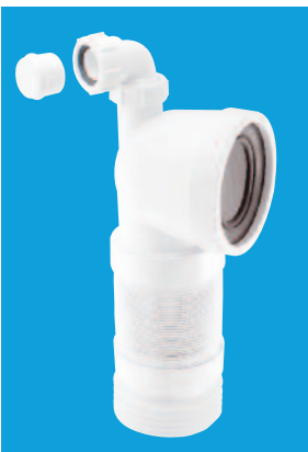
97-107mm Inlet 4"/110mm Outlet 1 1/4" Universal Vent Boss
