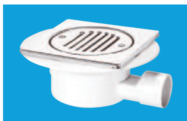
150mm Square Polished Stainless Steel Tile with removable Grid and Securing Screws 1½" BS EN 1329-1:2000 solvent weld horizontal outlet. Overall height 75mm
